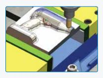
CAMWorks Milling Professional includes all the functionality in CAMWorks Milling Standard plus undercutting, fillet machining, NURB surface machining, and mill-turn with C, Y & B axis capabilities.
